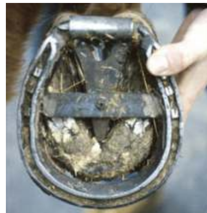
Figure 27. An all steel adjustable heart bar shoe. The heart bar is hinged at the base. The shoe is fitted with no pressure on the heart bar. Frog support is increased after nailing on by turning the grub screw (near the centre of the foot) with an Allen key.
